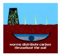
Experiments have been conducted with specific version of the wicking bed designed for carbon capture. The illustration shows a conventional wicking bed with a biobox which is regularly filled organic waste.
