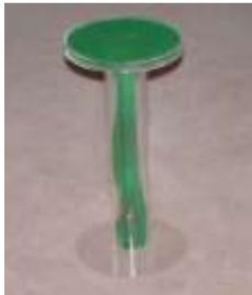
The decision when to irrigate must be based on standard irrigation practices, the simplest is to have an evaporation gauge as shown and irrigate when the accumulated evaporation reaches a certain level. This level can be easily determined by gradually increasing the accumulated evaporation until the plant shows signs of stress then cutting back the accumulated evaporation to between 50 and 80% of that required to cause stress.
