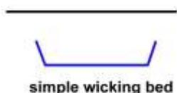
The simplest version of the wicking bed is shown. A trench is dug below the root zone and lined with an impermeable membrane (plastics sheet).
