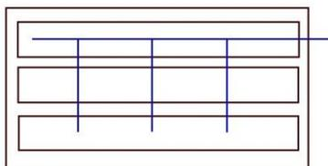
An alternative is to have just one pipe in the highest bed and as many overflow lines as needed. Overflow pipes can be added as needed after construction as often the flow characteristics of the organic waste may not be known at the design stage.
