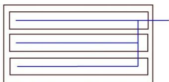
Water will not flow far through most soils (may be a metre or so). However water can flow a much greater distance through the porous organic waste (such as wood chips), may be 10 or even 20 metres. But for any greater lengths either a pipe or equivalent (such as bubble wrap) must be used. Pipes are the most expensive component in a wicking bed so this may be expensive.
