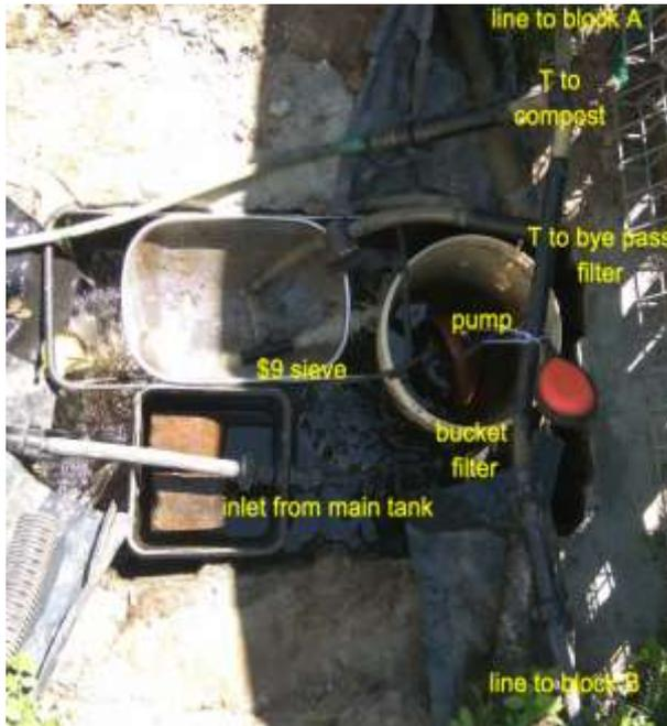
I therefore put a T in the line to create a bye pass filter. In hydraulics it is common to have a coarse in line filter and a much finer bye pass filter to generally clean up the oil. I am using exactly the same system with a coarse in line and a fine bye pass filter.
