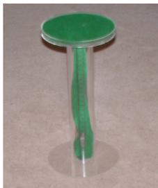
The decision when to irrigate must be based on standard irrigation practices, the simplest is to have an evaporation gauge as shown and irrigate when the accumulated evaporation reaches a certain level. This level can be easily determined by gradually increasing the accumulated evaporation until the plant shows signs of stress then cutting back the accumulated evaporation to between 50 and 80% of that required to cause stress.
